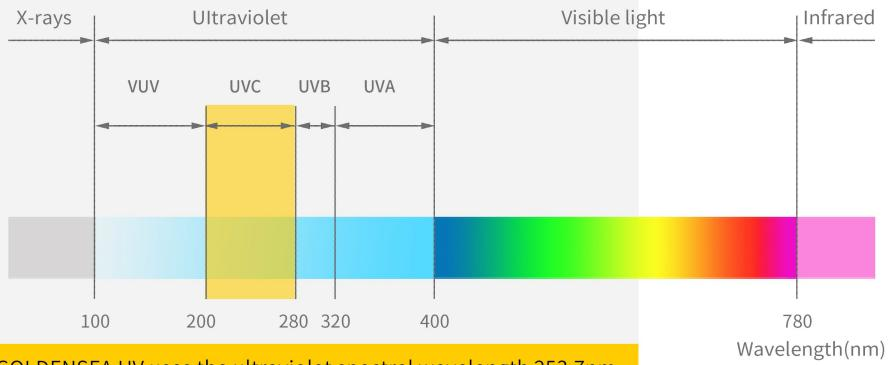
GOLDENSEA UV uses the ultraviolet spectral wavelength 253.7nm. This belongs to the short-wave UVC spectrum and is an efficient and better choice for disinfection!
